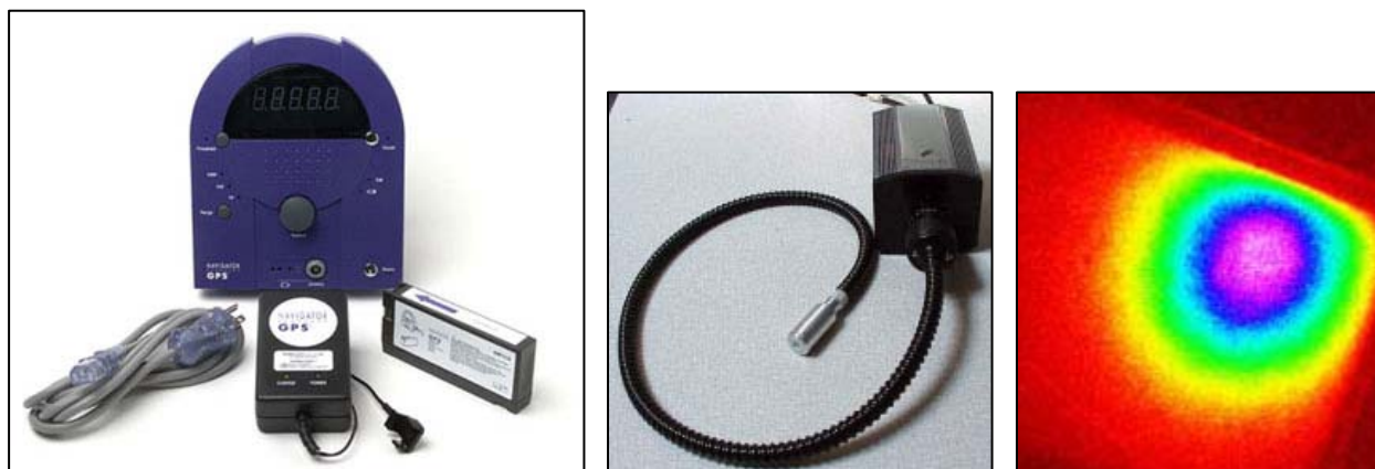
Figure 4. The Navigator base unit, shown in the left panel , is a multifunctional system used with various probes during surgery. One example of a probe, which is shown in the center panel , is the gamma-PET probe that enables surgeons to assess the location of a tumor's boundaries during surgery, rather than rely on images taken prior to surgery. The right panel is an example of an image of a tumor detected with the gamma-PET probe.
