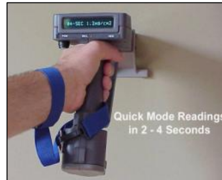
Figure 6. The LPA-1 XRF lead paint inspection system, pictured in the left panel with a portable data recorder, has three modes of operation. In the Quick Mode, the inspection system concludes the measurement as soon as a 95% confidence interval is reached, typically within 2 – 4 seconds.
