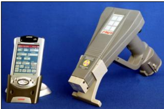
Figure 6. The LPA-1 XRF lead paint inspection system, pictured in the left panel with a portable data recorder, has three modes of operation. In the Quick Mode, the inspection system concludes the measurement as soon as a 95% confidence interval is reached, typically within 2 – 4 seconds.
